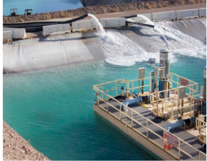
Barge pumps at Morenci transfer water from the tailings impoundment for recycling. The majority of our recycled water originates from reclaimed water captured at tailings facilities and leach pads.
